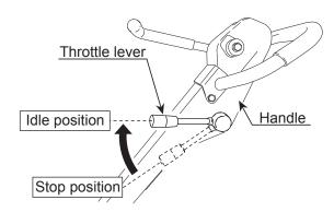
Figure 11. Throttle Lever (Idle Position)
